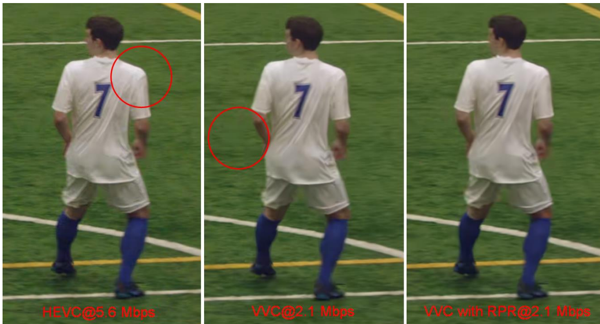
FIGURE 4: SCREEN SHOT FROM DECODED SEQUENCE FROM HEVC BITSTREAM (LEFT), VVC BITSTREAM (MIDDLE) AND VVC BITSTREAM WITH RPR (RIGHT). VVC WITH RPR DECODED PICTURES WERE UPSCALED TO THE ORIGINAL 4K RESOLUTION. HIGHLIGHTED AREAS POINT TO VISIBLE ARTEFACTS: HALO AROUND PLAYER'S SHOULDER (LEFT) AND SOFT PATCH IN THE ASTRO TURF (MIDDLE) SEQUENCE USED IN THIS TEST IS FROM [63].
